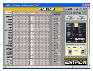
A PC or Laptop with RS232/RS485 converter and ENLINK for Windows may be used as a master device to communicate with EN1000 Series Controls.
